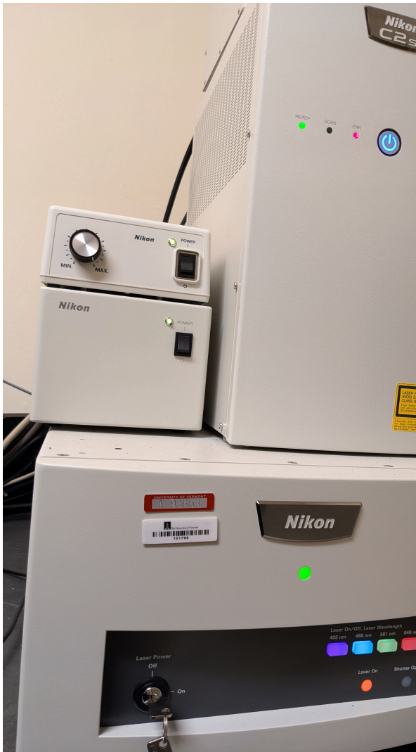
Figure 8: Switching on fluorescent light, shutter is closed
