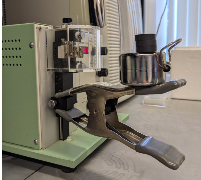
Figure 4: Puller weights on the machine
