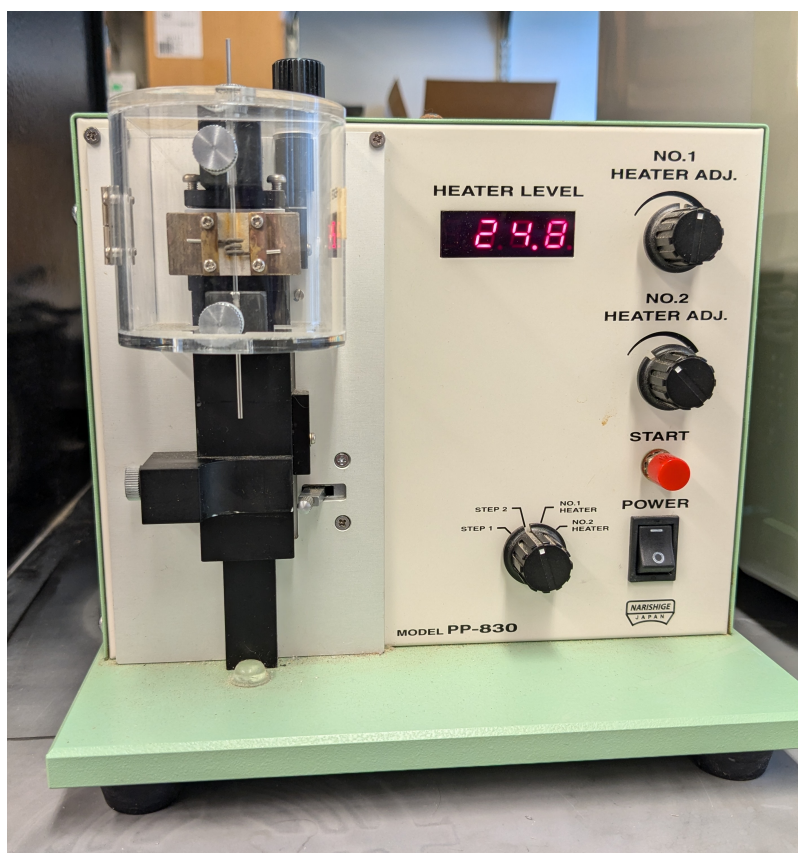
Figure 3: Correct capillary position
