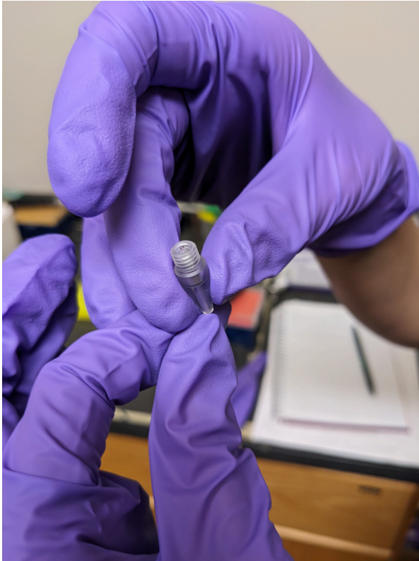
(a) Insert needle into needle holder, end first, make sure needle end is visible
